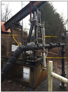
Figure 2.14: Gaseous tracer injection method.
