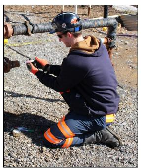
Figure 2.8: Tracer concentration sample being collected using Vacutainer.
