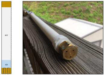
Figure 2.13: PVC assembly for PFT added to wellbore fluid.
