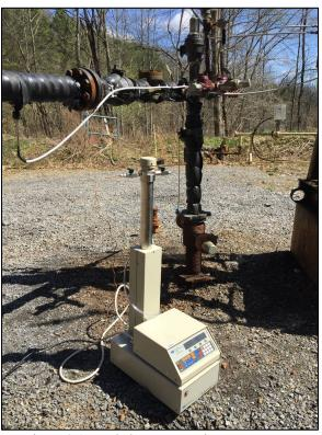
Figure 2.15: Teledyne Isco syringe pump.
