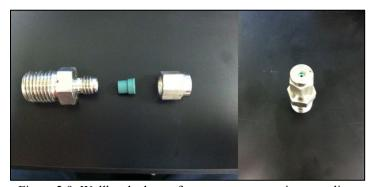
Figure 2.9: Wellhead adapter for tracer concentration sampling.
