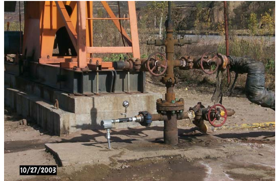
Well head with Downhole gauge packoff
